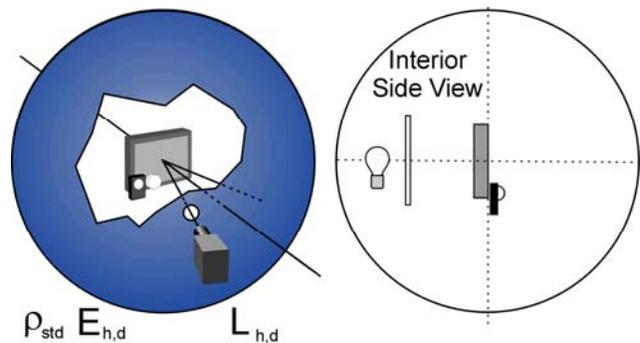
**Fig. 1.** Integrating sphere enclosing the display with illuminance meter and white diffuse standard. A baffled lamp is located behind the display. The measurement is made  $10^\circ$  from the display normal.
