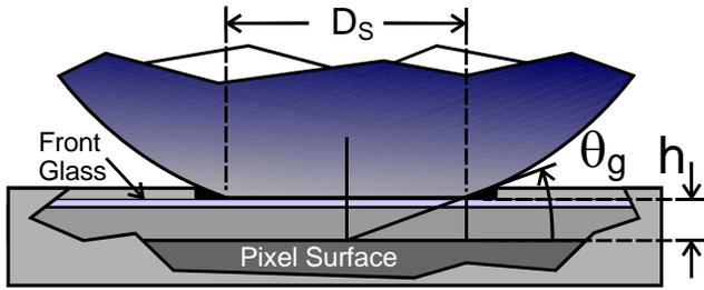
**Fig. 6.** Example of a sample port on the cover glass of a PDP where the pixel surface is offset from the front surface by a distance  $h$ .
