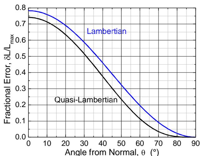
**Fig. 9.** Fractional error in luminance measurement for sampling port not being next to the pixel surface.
