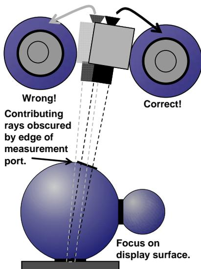
Fig. 3. Proper alignment of luminance meter with the measurement port is critical.
