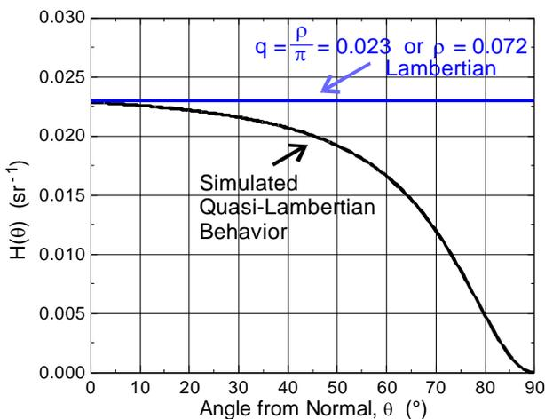
**Fig. 7.** Simulated analytical model of a BRDF,  $H(\theta)$ , for a quasi-Lambertian display with a front glass where the specular component is represented as an arrow at  $\theta = 0$ .
