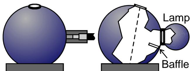
**Fig. 10.** Sampling sphere illumination possibilities using a fiber-optic illuminator (cutaway at left) or a satellite sphere with diffuser (right).
