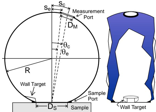
**Fig. 2.** Sampling sphere. Luminance measurements are made through the measurement port.
