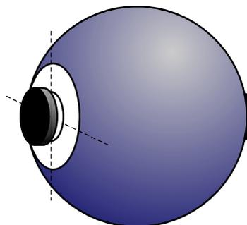
Fig. 4. White standard placed in the plane of the sample port for calibration of the wall target.
