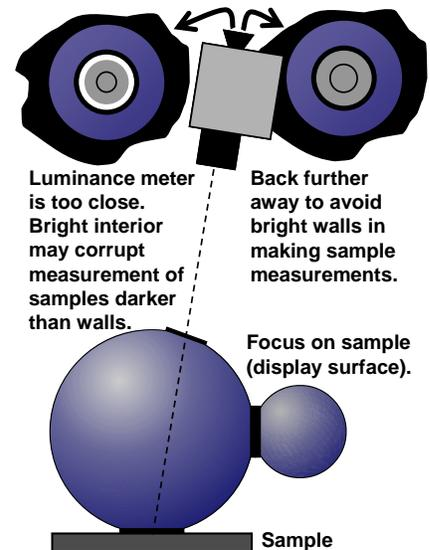
Fig. 5. Position of luminance meter sufficiently far away from measurement port to avoid veiling-glare corruption of darker samples.
