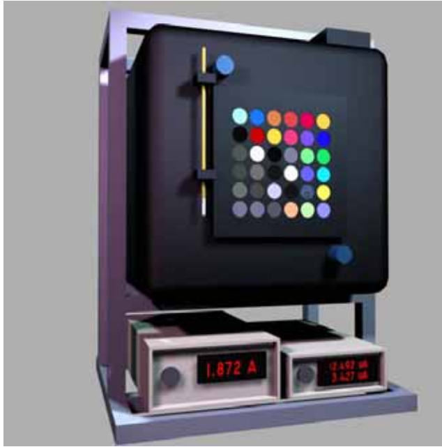
Fig. 1 Each DMATS unit will consist of a uniform illumination source with a suite of optical targets mounted in a faceplate, power supply, monitoring devices, and a laptop computer for automatic data logging.
