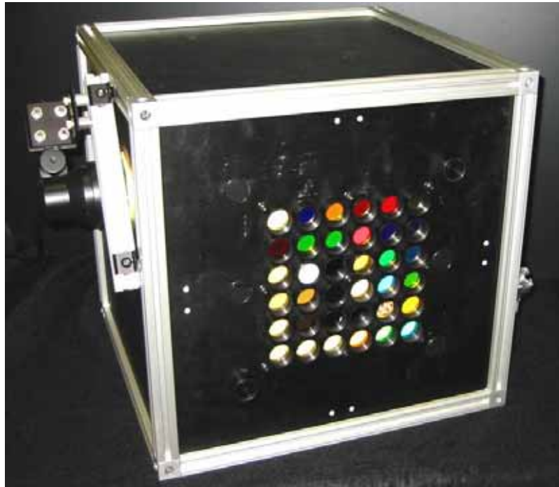
Fig. 3 Current “ruggedized” DMATS constructed of extruded aluminum components, expanded PVC shell, and polystyrene box liner. Exterior dimensions (w x h x d) are 44 cm x 43 cm x 43 cm.
